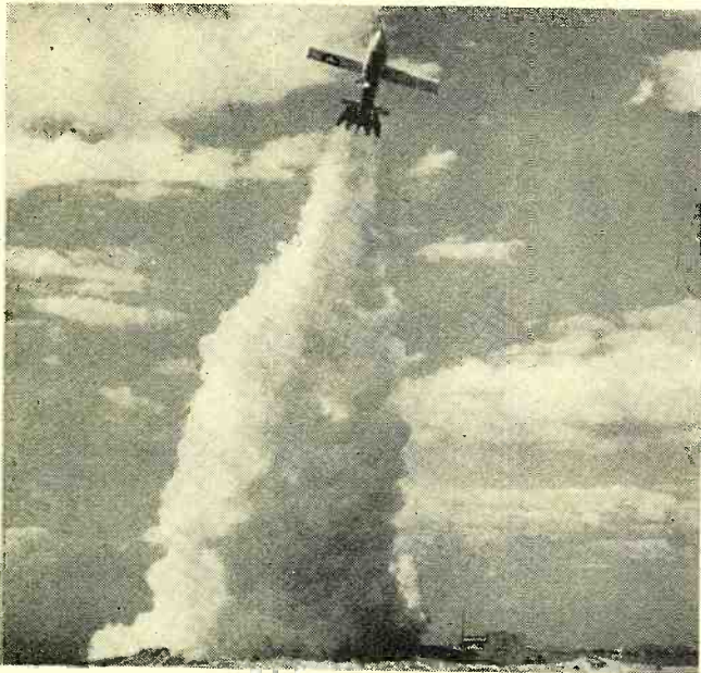
Guided missile roars into the air with the aid of four Mons-auto rockets. After expiration of the thrust of 40,000 pounds, the rockets and sled will fall free and the "Loon" will head out over the Pacific to its target.
