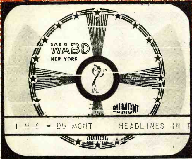
Fig. 1. (Left) White streaks appearing in image are due to faulty ignition systems of cars and trucks passing near antenna site. Fig. 2. (Above) Effect indicates overloading of receiver input, loss of sync control, and some leakage into the video output circuit. Curvature of lines suggest that part of interference may be due to powerful nearby FM stations.
